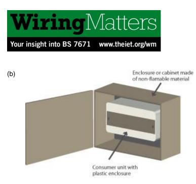
There is no published definition for the term 'non-combustible' that aligns with the intent of Regulation 421.1.201. However, as stated in Note 1 to the regulation, ferrous metal, such as steel, is deemed to be an example of a non-combustible material.
